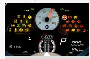
**The Advanced Dashboard** displays Engine and PTO speeds, service intervals, fuel consumption, distance travelled, area worked, oil temperature and tractor hours, Engine memorised speed and service information.
