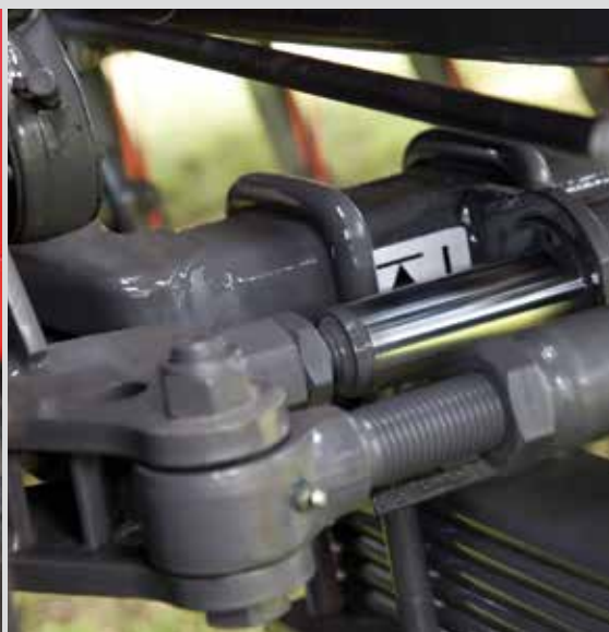
Rear axle hydraulic steering lock.
