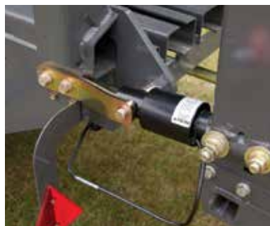
Highly accurate load cells for the Integrated Bale Weighing System.
